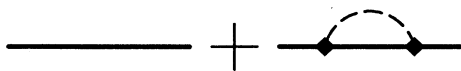
FIG. 7. Expansion for the partition function in u_0 up to one loop. The dashed line represents the excluded volume interaction, which can be characterized by the interaction parameter u_0 , between the two points specified by the diamonds.
